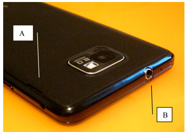
Figure 3. Auxiliary affordances of a mobile phone. A: back cover removal slot (maintenance); B: headset jack slot (aggregation).
