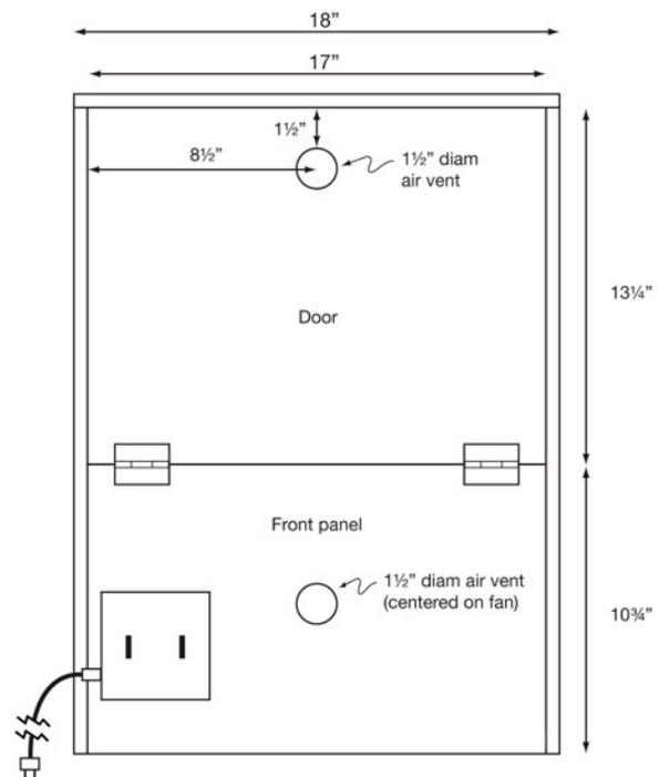
Figure 3. Front view cross-section of dehydrator construction
