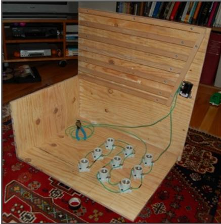
4. Next, screw the left side panel and front panel to the base (figure 7). I also used wood glue (Titebond) to make the joints stronger.
