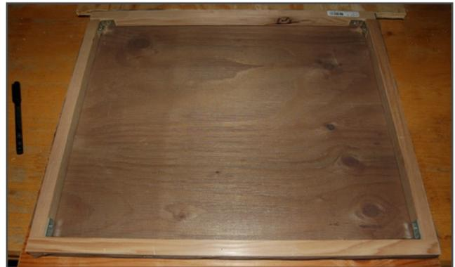
13. To build drying trays like that shown in figure 9, I used 1 × 1-inch nominal (¾ × ¾-inch actual) pieces of wood, cut to the lengths indicated in figures 3 and 4. Use L-brackets to re-inforce the corners of the trays and prevent twisting of the wood pieces (figure 10). Lay the 1 mm mesh nylon screen over the finished tray frame, and cut the screen around the tray frame, adding 1 ½ to 2-inches of screen to the overall dimensions.
