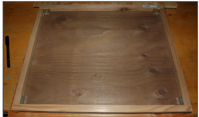
Figure 9. Completed drying tray, assembled from ¾ × ¾-inch wood pieces and 1 mm mesh nylon screen
